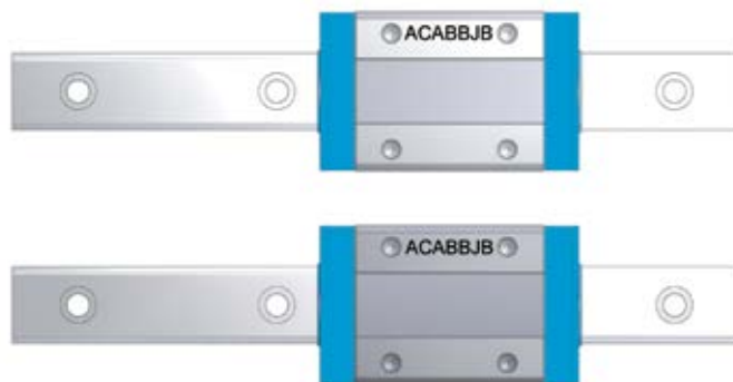
Figure 3.4 Marking the main and auxiliary guide
