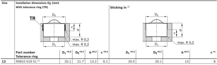
1) Made from corrosion-resistant steel 1.4310
