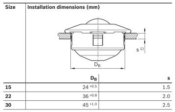
1) Minimum thickness of the mounting plate
