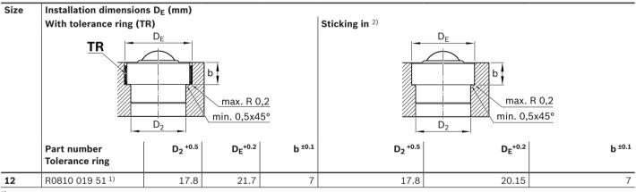
1) made from corrosion-resistant steel 1.4310
